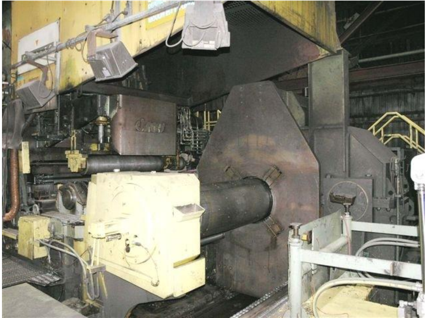
TENSION REEL #1 W/ OUTBOARD BEARING SUPPORT 24" DIA MANDREL (610mm) 4000HP MOTOR DC (2 x 2000HP) (2 x 1500Kw) 395 / 1000RPM – 730v
